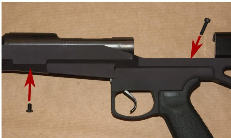
2. Engage slightly (!) by 2-3 turns the M6x10 forward main screw. It should fit without forcing.
