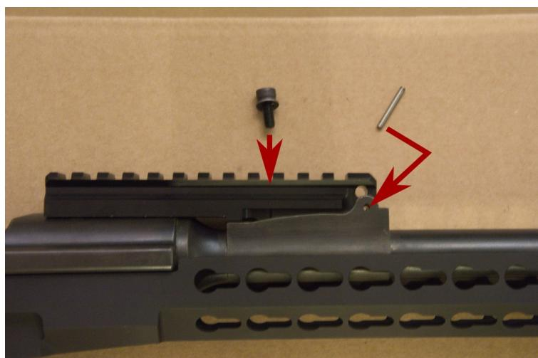
6. Screw the M5x12 screw into the nut through the rail. Tighten (recommended torque 8.5 Nm).
