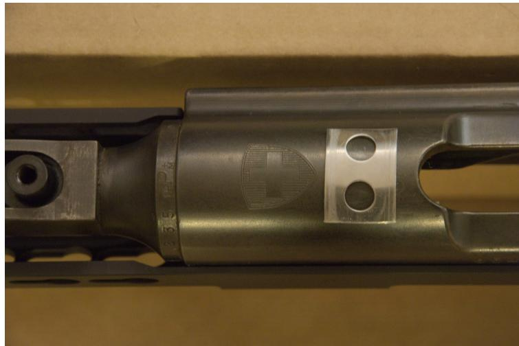
5. Place the rail on top of the nut (and on top of the inclination insert, if there is one) and insert the rail in the sight housing, so that the pin holes of the housing and the rail coincide. Fix the parts together with the sight pin.
