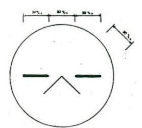
The thickness of the reticle crosshairs is  $0.5_{\,0/00}$ . The thickness of the auxiliary crosshairs is  $2_{\,0/00}$ . The visual field of Model 41/42 (magnification 1.8X) measures  $125_{\,0/00}$ ; The visual field of Model 31/43 (magnification 2.8X) measures  $80_{\,0/00}$ .
