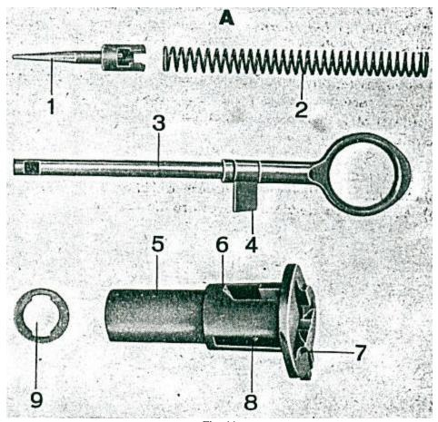
Fig. 11 Firing Mechanism
