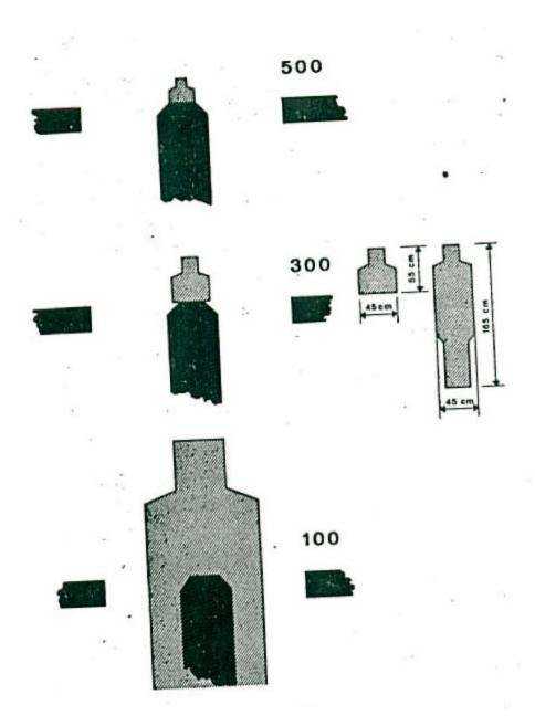
$$\operatorname{Fig.28}$$  Method for gauging field targets at distances of 100, 300 and 500 m
